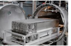
High Temperature and High Pressure Cleaning Device
